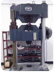
Tensile Strength Testing Machine
